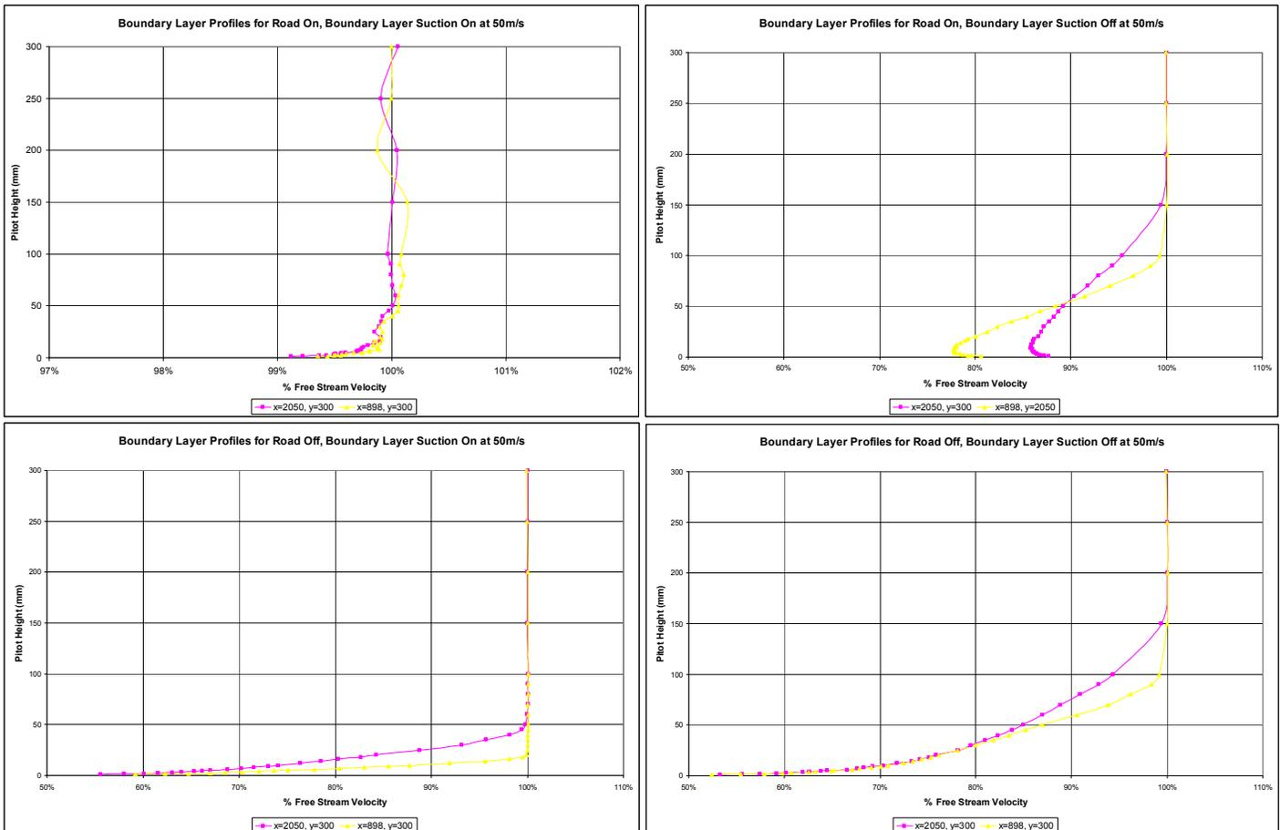
Figure 15 a-d: Boundary Layer Profile variance between x=2050 and x=898.
