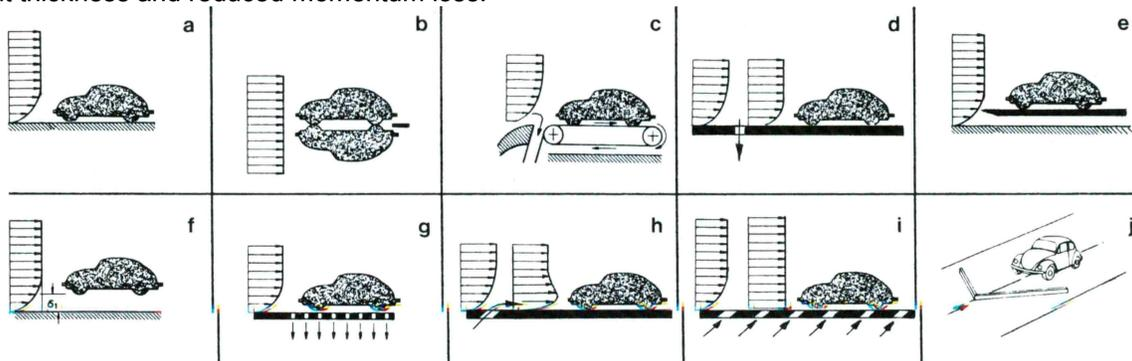
Figure 4, a-j: Varying forms of boundary layer control. Source [1]
