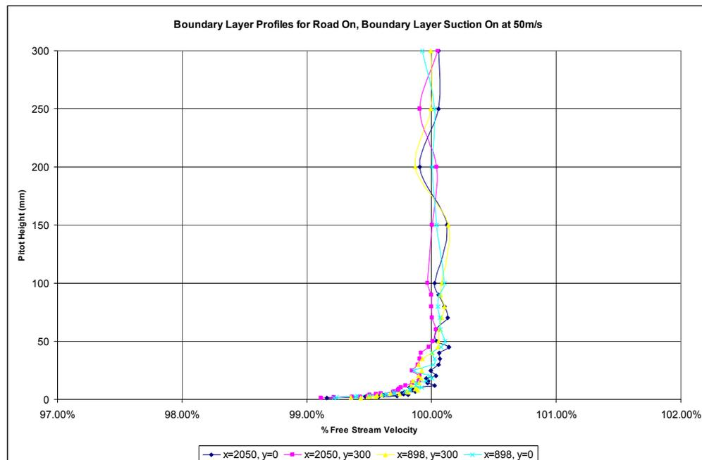
*Figure 8:* Boundary layer profiles at 50m/s for road on and boundary layer suction on
