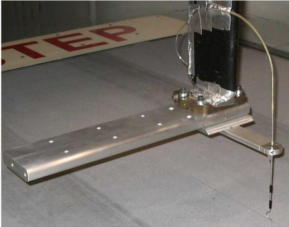
*Figure 6:* Pitot tube mounted on sting at position  $x=2050$ ,  $y=0$
