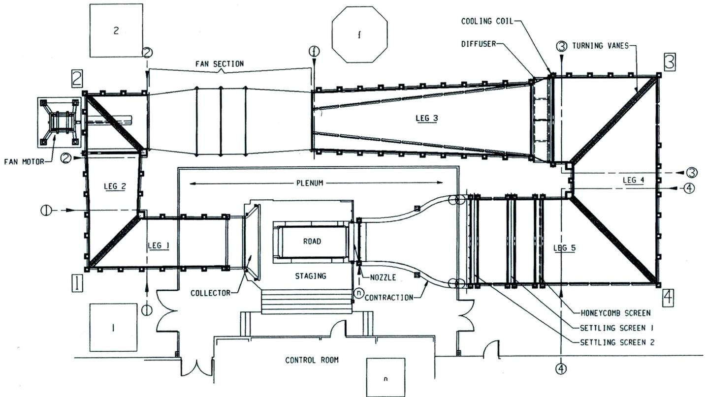
Figure 3: Schematic diagram of the ARC wind tunnel. Source ARC
