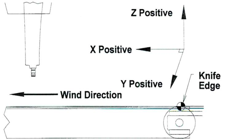
*Figure 7:* Working section coordinate system
