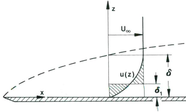
Figure 5: The boundary layer profile. Source [1]
