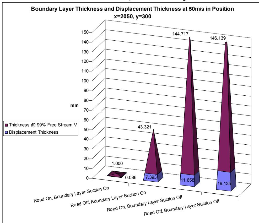
Figure 9: Boundary layer thicknesses and displacement thicknesses,  $x=2050$ ,  $y=300$
