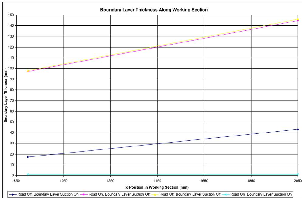
Figure 10: Boundary layer thicknesses at y=300 and varying x
