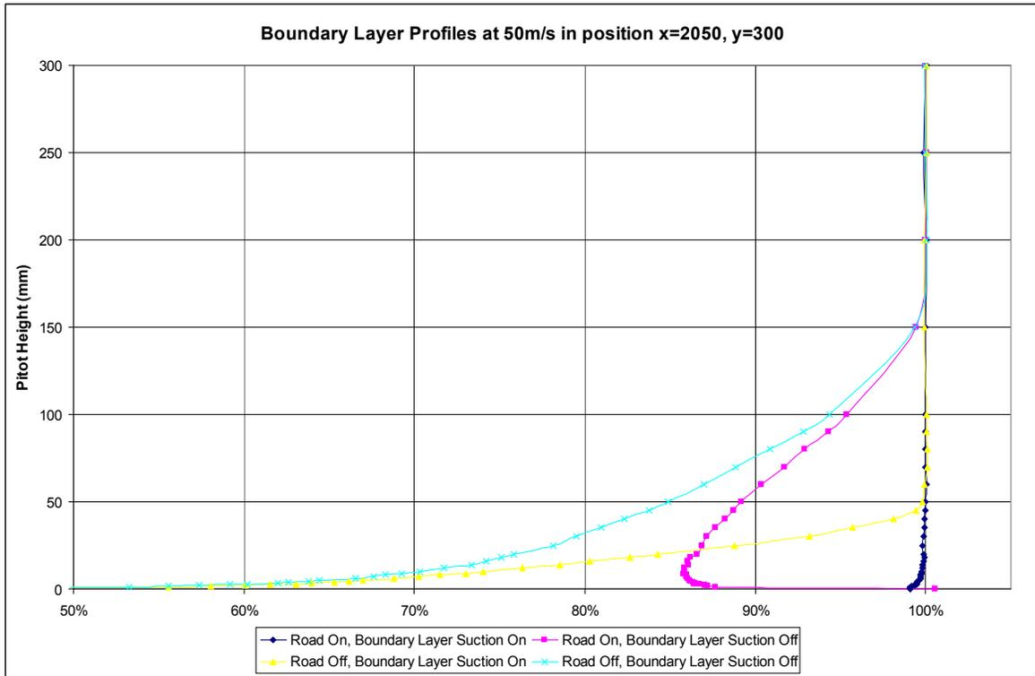
Figure 1: Boundary layer profiles measured at position x=2050, y=300 for each case at 50m/s.
